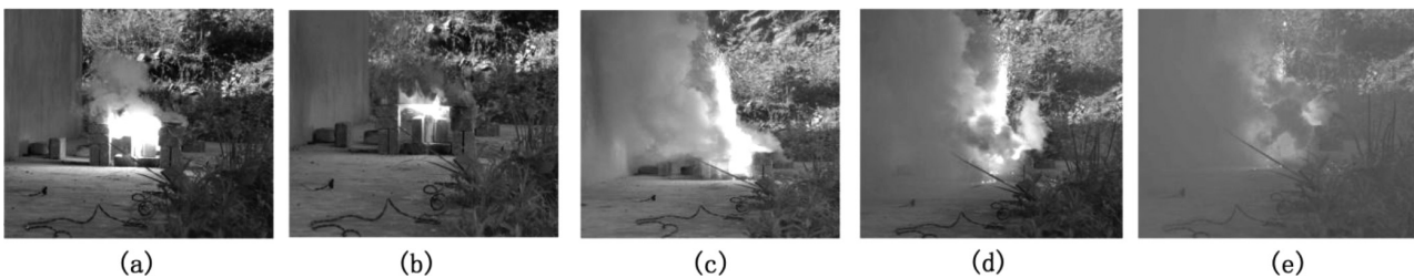
Figure 2: The Al/MnO 2 pyrotechnic cutting agent combustion experiment
