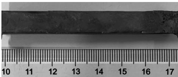
Figure 3: The prepared samples of CC-M f /Al and CU-M f /Al composites
