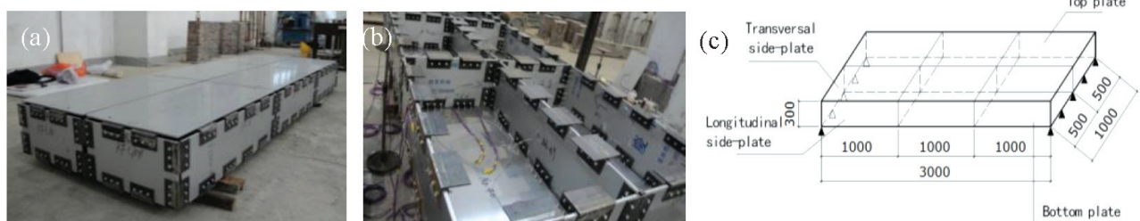
Figure 2: Full-scale specimen overview: a) the total appearance, b) internal structure, c) geometrical dimensions
