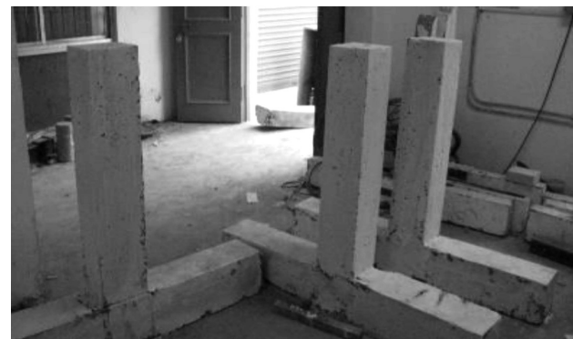
Figure 2: Casted beam-column specimens
