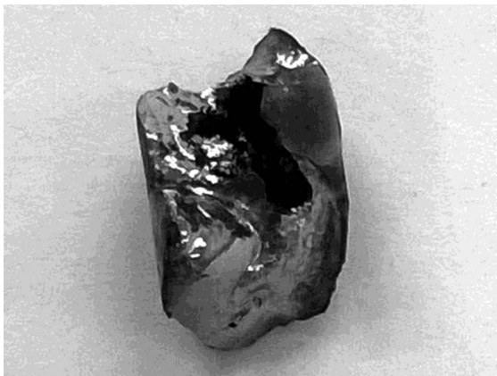
Figure 9: Morphology of NiTi46 (in mass fractions, (w%)) compressed powder mixture reactively sintered 900 °C for 120 min
