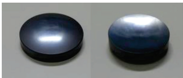
Figure 3: A silicon single-crystal lens obtained from a CZ silicon disk (Φ22 × 4 mm) by molding at around 800 °C (actual sample temperature), which is about 600 °C lower than the melting temperature, by using an SPS system
