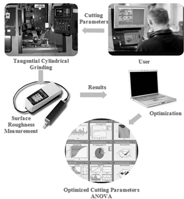
Figure 2: Flowchart for optimizing the cutting parameters in tangential cylindrical grinding process
