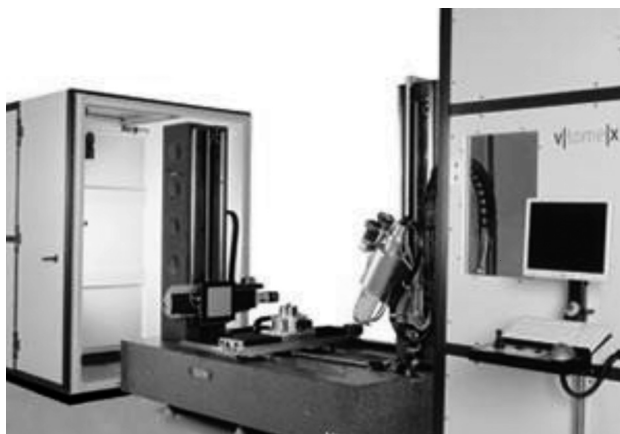
Figure 4: Microscope station GE Phoenix v|tome|x L 240 16 Slika 4: Mikroskopska postaja GE Phoenix v|tome|x L 240 16
