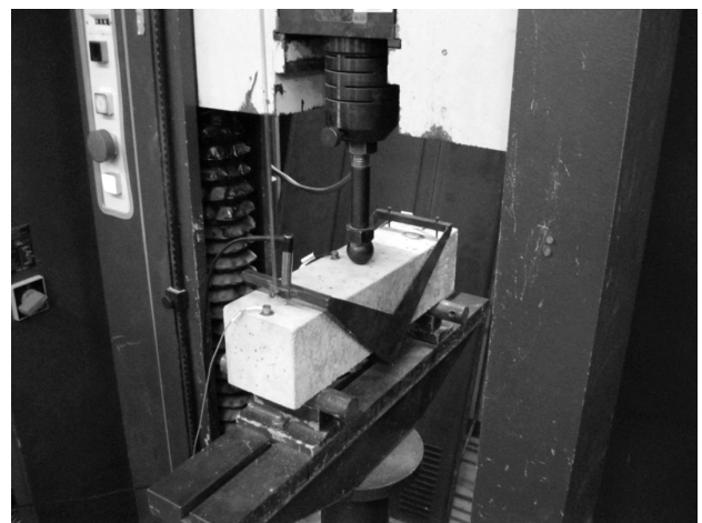
Figure 2: Fracture-test configuration in testing machine
