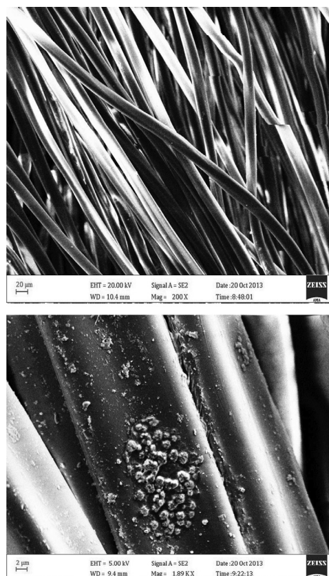
Figure 3: SEM micrographs of samples: a) polyester-filament yarn, b) nano-silver-coated polyester-filament yarn
