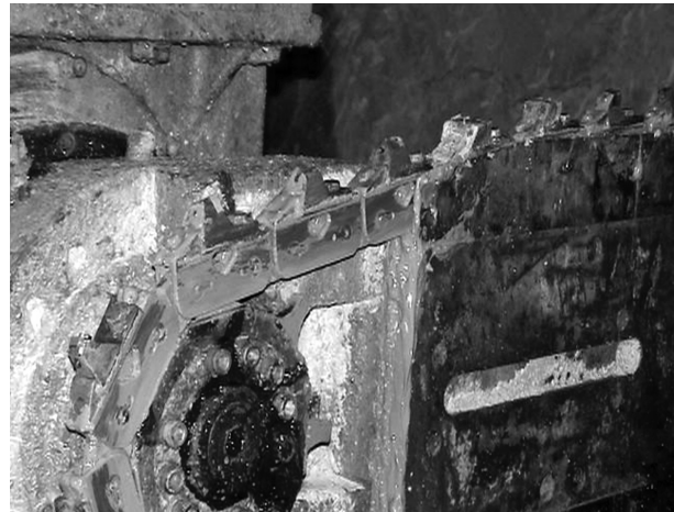
Figure 7: Detail of the chain and arm/blade of the chainsaw machine Slika 7: Detajl verige in zobnika roke/meča verižne žage
