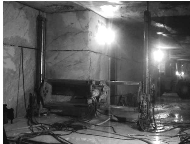
Figure 1: Column-driven chainsaw machine Fantini G.70 on the location in the Hotavlje I quarry
