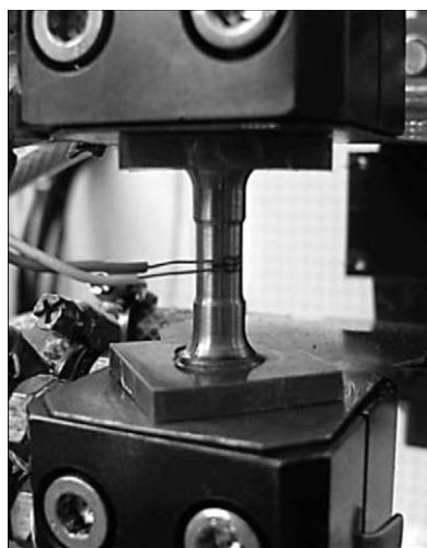
Figure 1: Specimen mounting in the thermomechanical simulator
