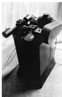
Figure 5: a) Schematic view of the contact pair (pin and disk) and b) image of Tribometer TPD-93
