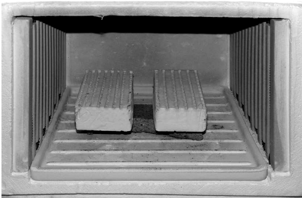
Figure 6: Thermal treatment of plaster investment to burn the polymer foam
