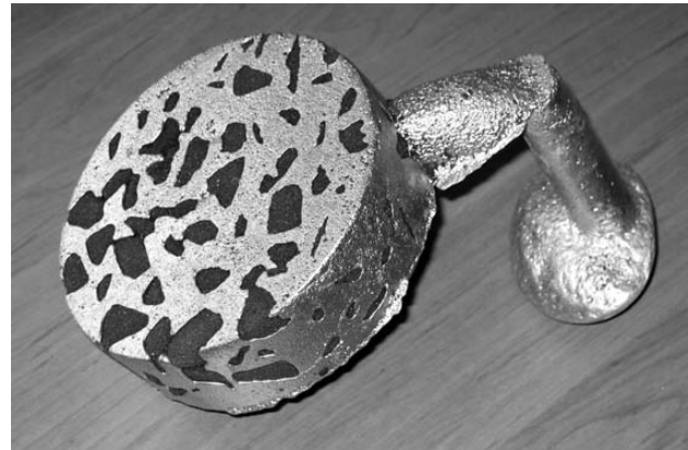
Figure 8: Casting made of AlSi10MgMn with remaining precursors
