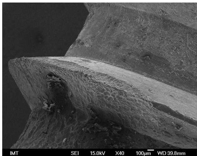
**Figure 7:** Corroded screw (SEM)
