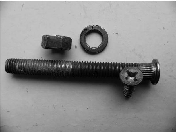
**Figure 3:** A nut, a spring washer, a structural bolt of the stairs and a cross-head screw, all covered with rust
