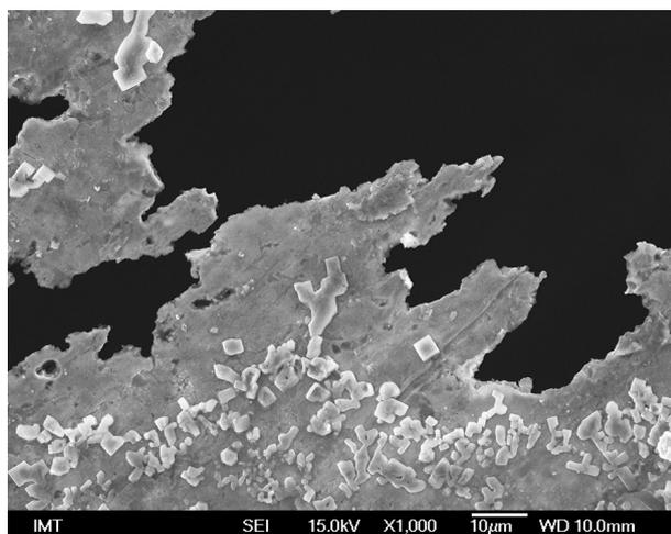
**Figure 9:** Remains of NaCl around a crevice-corrosion cavern (SEM)
