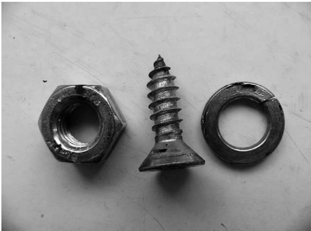
**Figure 4:** Corrosion-damaged structural components after cleaning with ultrasound
