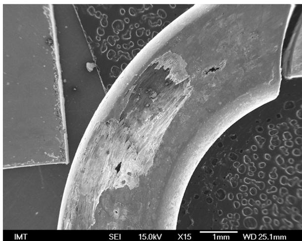
**Figure 8:** Crevice corrosion of a spring washer (SEM)
