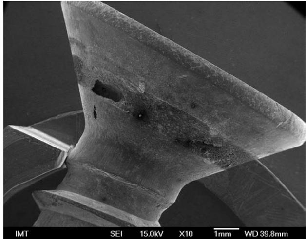
**Figure 5:** Screw damaged by crevice corrosion (SEM)
