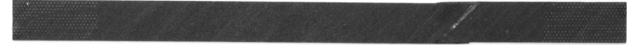
Figure 2: Fractured [\pm 45]_{2S} specimen. The position and orientation of the cracks is emphasized Slika 2: Prelomljen vzorec [\pm 45]_{2S} . Poudarjena sta položaj in orientacija razpok
