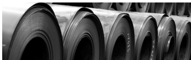
Figure 1: Coils of cold-rolled, non-oriented electrical steel 5 (Acroni, d. o. o., Jesenice)
