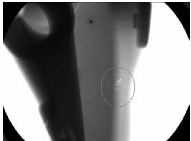
Figure 5: X-ray picture of shrinkage porosity in one of the components
