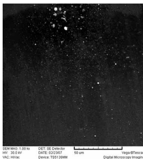
Figure 8: The traces of deposited plasma visible on the smooth glassy carbon plate Slika 8: Na gladki steklasti ogljikovi ploščici so vidni sledovi nanosa plazme
