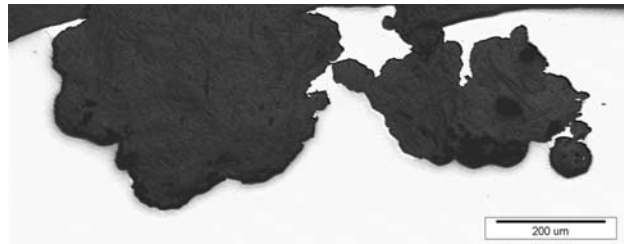
Figure 5: Micrograph of cross-section of the corrosion pit on the bent edge. Local corrosion advanced deep into the material of the case wall Slika 5: Posnetek preseka korozijske jamice na upognjenem robu. Lokalno je korozija prodrla globoko v material stene ohišja
