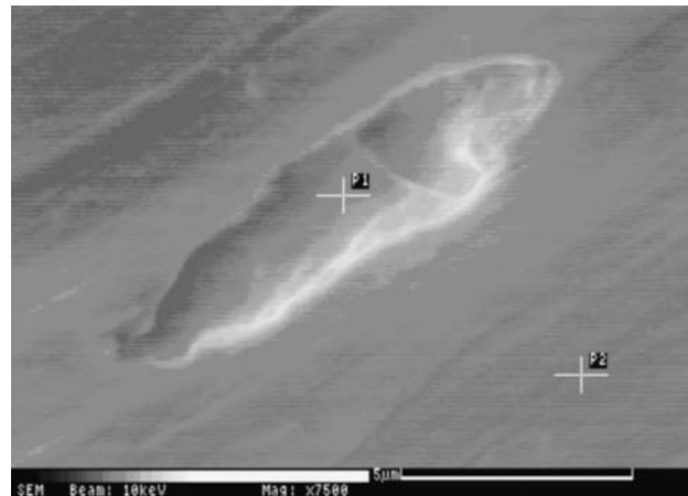
Figure 9: Surface with corrosion pit. At the points P1 and P2 the AES analyses were performed. The presence of Cl was detected only in the pit. SEM
