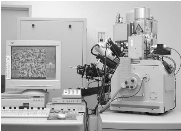
Figure 1: FEI Strata Dual Beam FIB in NCEM LBNL, University of California, Berkeley
