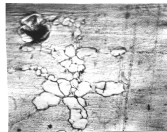
Figure 8: Microstructure of the surface of specimen 3-0 after 100 cycles (150–900 °C)
