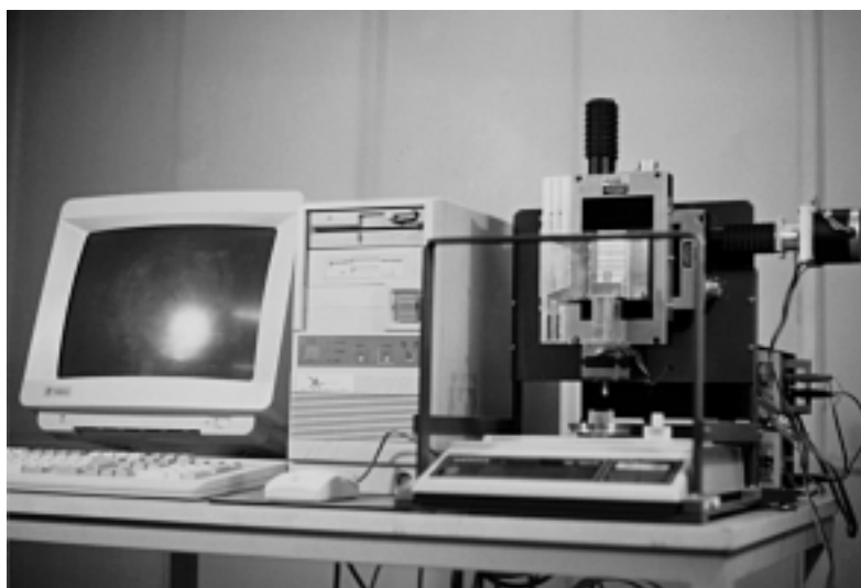
Slika 1: Računalniško vodeni sistem za merjenje kontaktnih karakteristik U_c(I) Figure 1: Computer supported system for measuring the contact characteristics U_c(I)
