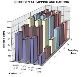
Figure 1: Change of the nitrogen content from tapping to casting of different steel grades with carbon content between 0.04 and 0.30%; 1 - converter, 2 - laddle before treatment, 3 - laddle after treatment, 4 - after casting 25% of melt, 5 - after 50% and 6 - after casting 75% of melt
