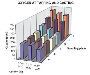
**Figure 2:** Change of the oxygen content from tapping to casting of different steel grades with carbon content between 0.04 and 0.30% **Slika 2:** Sprememba vsebnosti ogljika od šarže do šarže ra različna jekla z ogljikom med 0.04 in 0.3%
