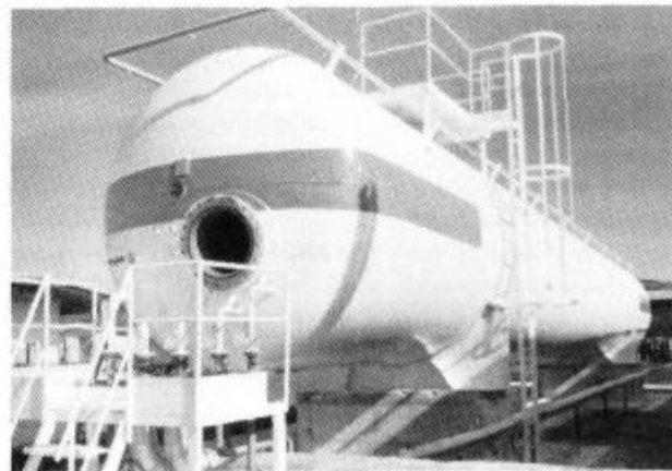
Slika 1: Horizontalna stabilna tlačna posoda prostornine 150 \text{ m}^3 Figure 1: Horizontal stable pressure vessel of volume 150 \text{ m}^3
