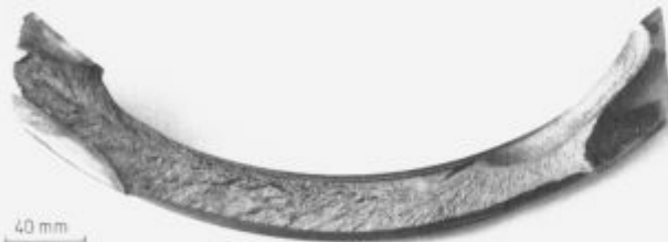
Figure 4: Fracture of the blade 447 extracted from the disc after the break down. The initial crack is on the left side.
