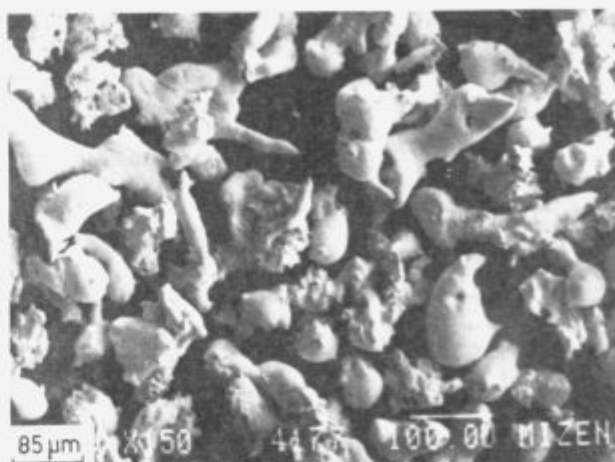
Figure 8: SEM micrograph of Au-Cu water atomized powder with irregularly shaped (tear drop and ligamental) particles. Slika 8: REM posnetek vodno atomiziranega prahu na osnovi Au-Cu z delci nepravilne (vlaknaste in kapljicaste) oblike.
