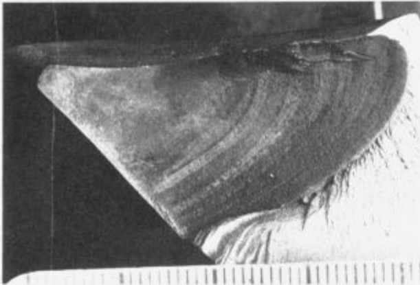
Figure 2: Surface of a crack with areas with and without fatigue striations.
