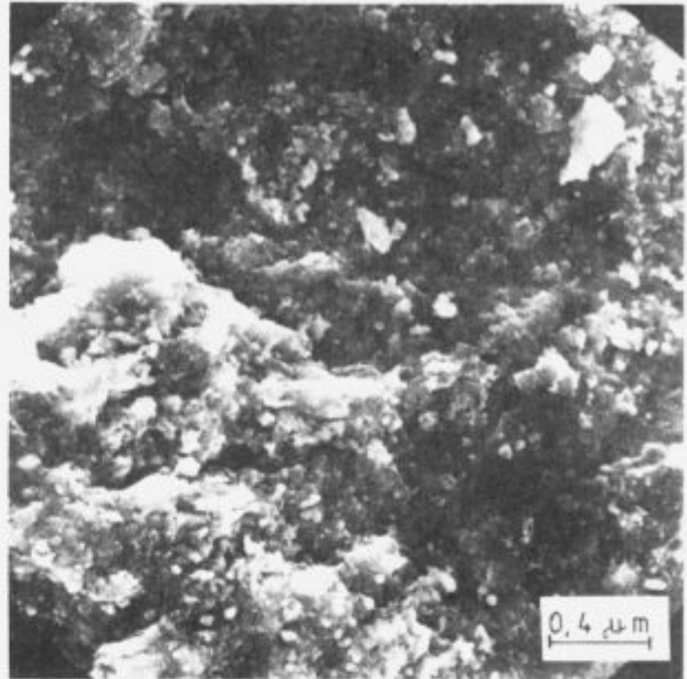
Figure 5: Damaged running surface - parts of oxides, stickers of metals... (unsurfaced running wheel)
