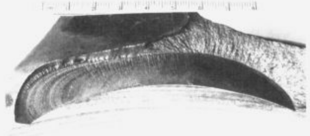
Figure 6: Surface of the crack on the blade on fig. 4.
